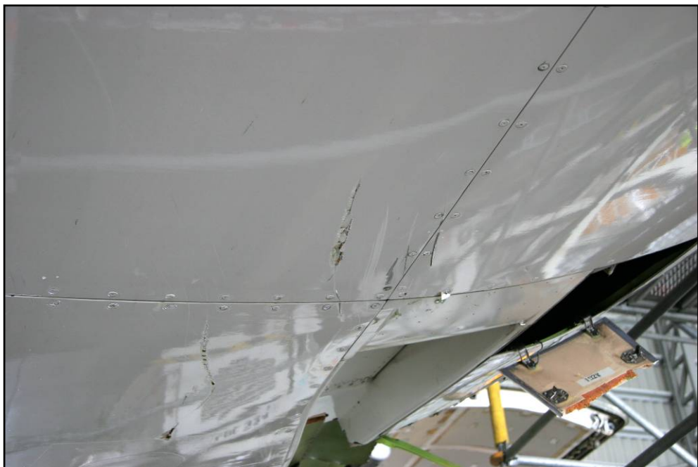
Figure 6: Panel damage to the rear of the rupture site
