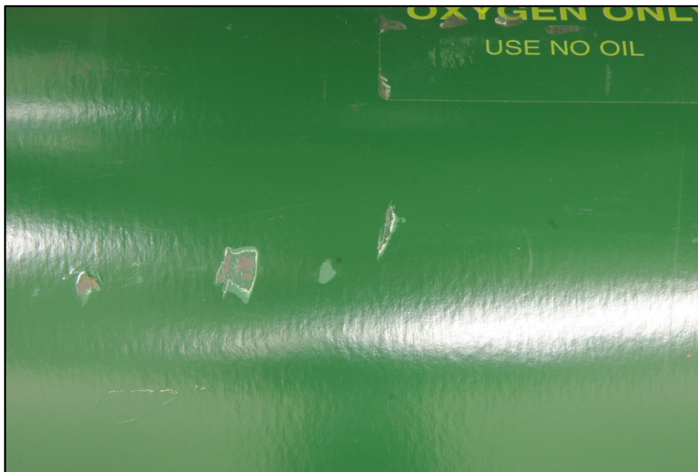
Figure 29: External surface marks on exemplar cylinder SN: 535598
