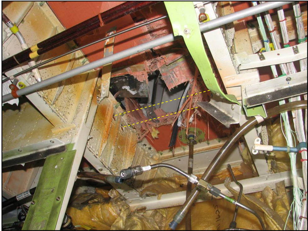
Figure 19: Door frame damage, green paint smear and rotated R2 door handle
