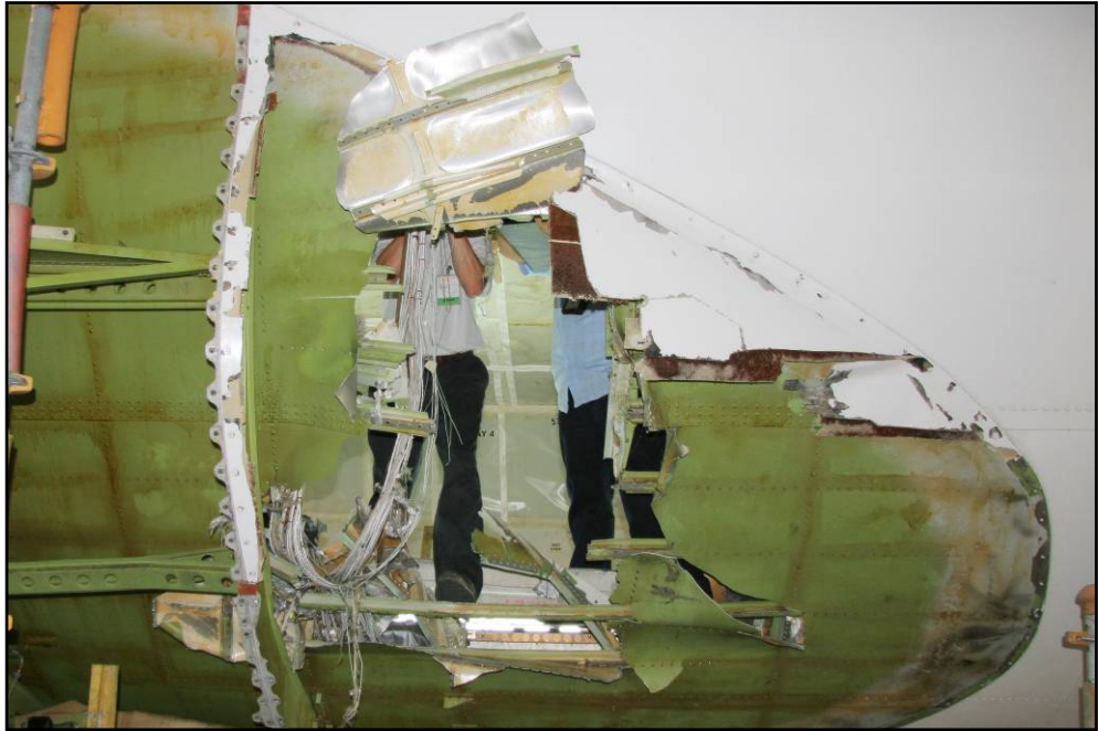
Figure 4: Sharply folded area of fuselage skin
