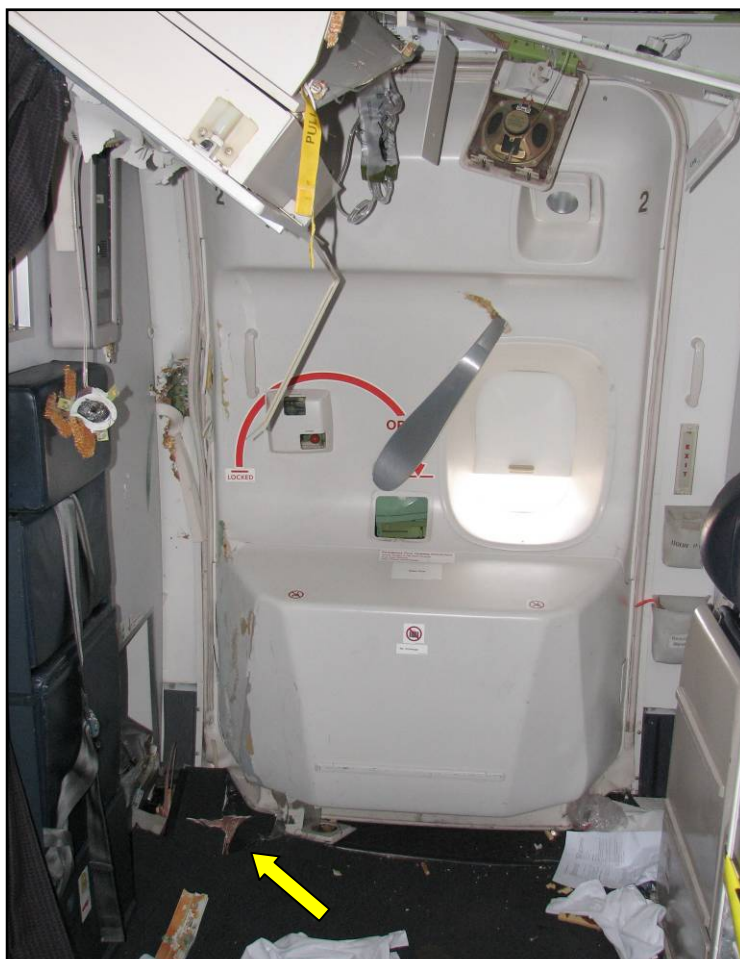
Figure 17: Interior of R2 door and cabin – location of floor hole arrowed
