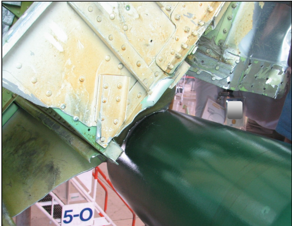
Figure 6: Panel damage to the rear of the rupture site
