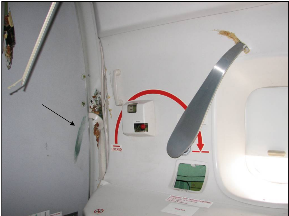
Figure 19: Door frame damage, green paint smear and rotated R2 door handle
