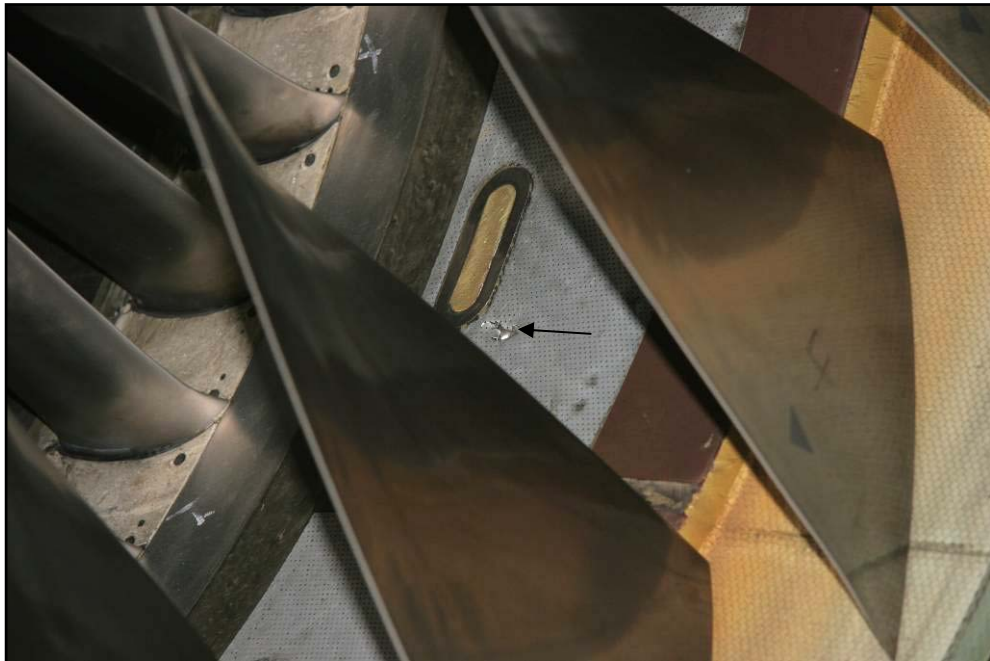
Figure 15: Damage to acoustic lining (arrowed) behind the number-3 engine fan
