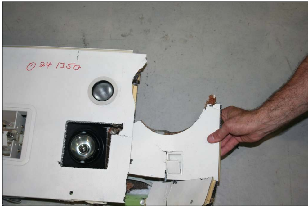
Figure 23: Panel with cut-out placed against another oxygen cylinder to illustrate the conformance in diameter
