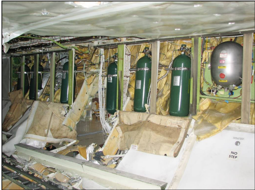
Figure 9: Fuselage rupture coincident with mounting position of the number-4 oxygen cylinder
