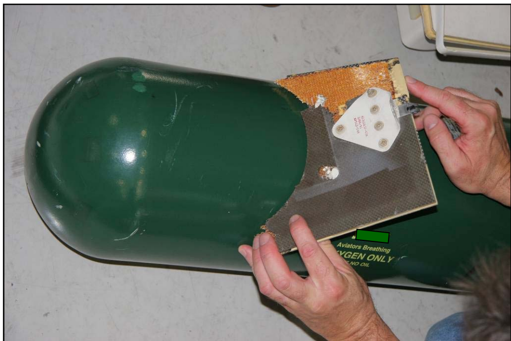
Figure 23: Panel with cut-out placed against another oxygen cylinder to illustrate the conformance in diameter
