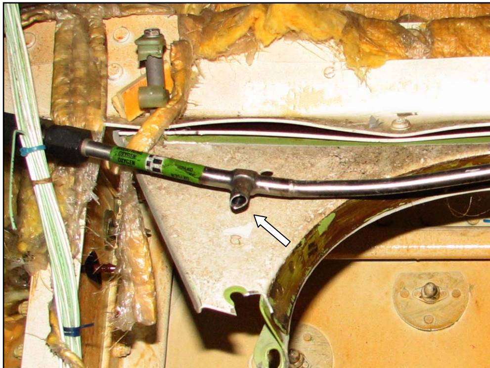
Figure 14: Number-4 cylinder overpressure discharge line fracture (arrowed)
