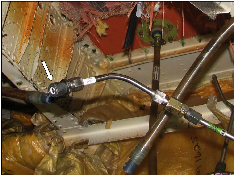
Figure 13: Number-4 cylinder service line fracture (arrowed)
