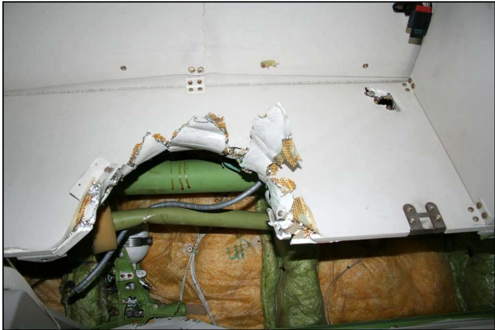
Figure 24: Semi-circular damage in partition of compartment above R2 door
