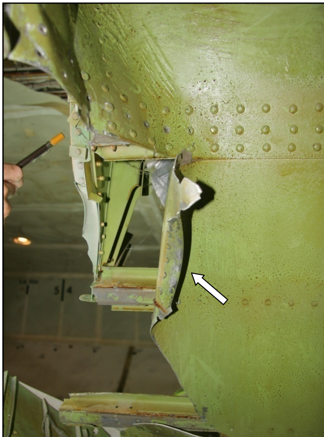
Figure 4: Sharply folded area of fuselage skin
