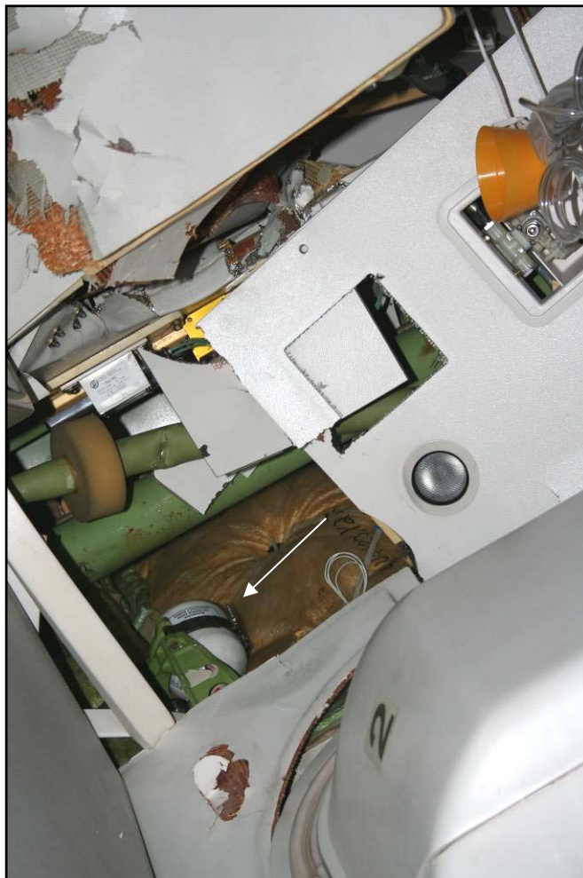
Figure 21: Damage above R2 door, exposing the EPAS cylinder (arrowed)
