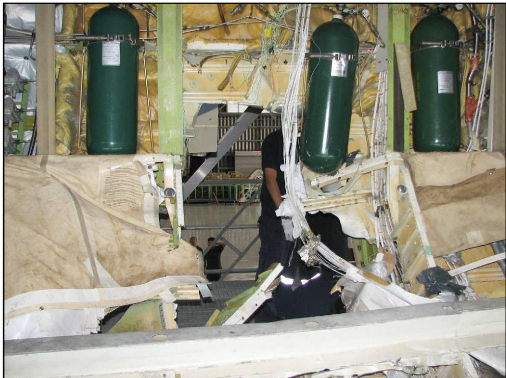
Figure 9: Fuselage rupture coincident with mounting position of the number-4 oxygen cylinder
